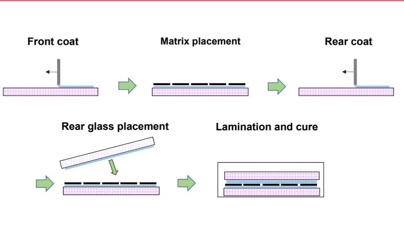
Figure 6. Encapsulation process using PV-6212 silicone encapsulant for glass-glass modules.
