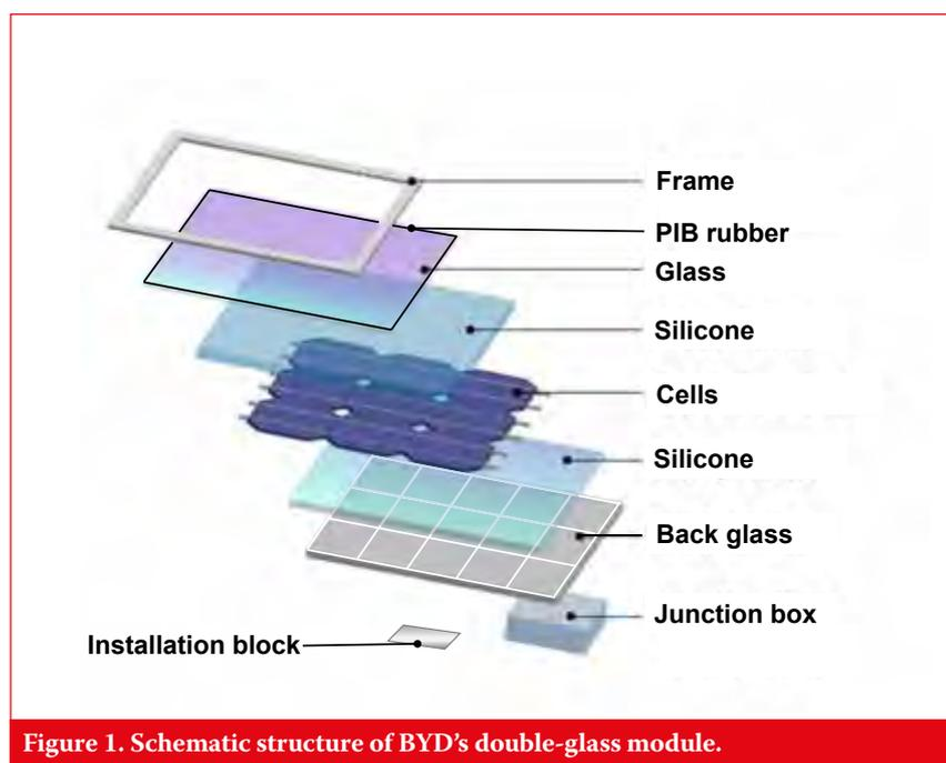
Figure 1. Schematic structure of BYD's double-glass module.
