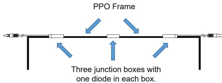
Figure 2. Detail of BYD's double-glass PV module design, highlighting the frame and the edge junction boxes.
