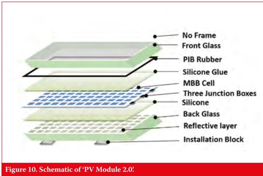
**Figure 10. Schematic of 'PV Module 2.0'.**
